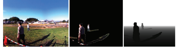
Figure 9: Depth estimation using a spherical vision camera. The image on the left is the original frame. The middle image shows segmented foreground. The one on the right is the estimated depth map. The shadow in the last image is considered to be foreground and not separated yet.
